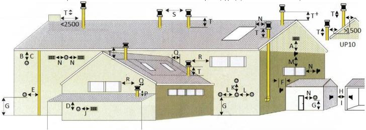
Horizontal Terminals Shall Not Be Located: Discharging into any road, track, thoroughfare, walkway or property boundary, to any play area/playing field, seating area or area where public gatherings take place. Where a surface or building element that may be adversely affected from plume condensates. Where vehicles may be parked unless separated by at least 1800mm.
